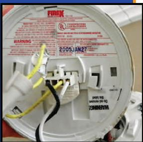
The reverse side of the smoke detector should list the year of manufacture.
